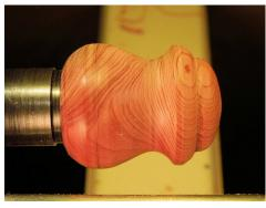
Round the base from the lower widest point down to the edge of the Forsner hole.
