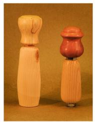
I use a hand piece to hold the stopper knob during the finishing process. The one on the left has a  $\frac{1}{2}$ " hole to hold the dowel. The one on the right has a  $\frac{3}{8}$ -16 bolt to hold the threaded knob.
