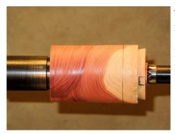
The stopper block has been turned downed to 1 3/8" to match the largest diameter of the finished knob.
