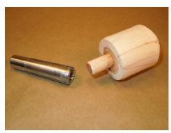
I used medium CA to glue the dowel into the block and sealed the Forsner cut surface with thin CA.
