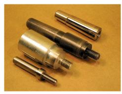
I use a collet to hold the dowel on the a cork or silicone stoppers. The cork stopper uses a 3/8" collet. The silicone stoppers from Peachtree uses a ½" collet.
