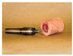
With the bottle stopper inserted fully into a bottle, I measured the length of the stopper above the bottle. I subtracted 1/16" from this number and bored the Forsner hole to that depth. The bottom of the Forsner hole is a finished surface so I sealed it with thin CA.
