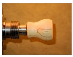
Cut a small taper on the base edge of the block.
