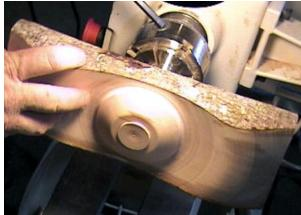
shape will be the feet on which the bowl ultimately rests. The inner curve forms a hemispherical central base that mates with the hollow vessel to be turned on the top side. He turns a tenon on this base which will be used to hold the piece when it is reversed for turning the upper surface of the bowl. When turning this shape it is very important to roll the gouge to almost a vertical position when approaching a change in curvature to prevent the lower cutting edge from catching.
