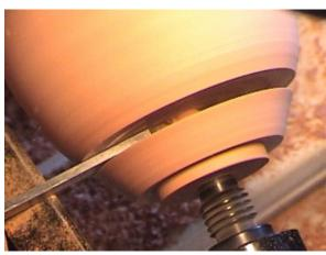
Bruce chose to demonstrate two different turning techniques at our meeting. The first was his method for turning a hollow form through reverse chucking and the second was illustrating how to turn a winged hollow form.
