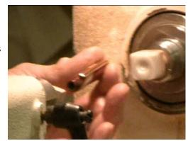
**6. Offset Turning** Offset turning can be done on short pieces with just the chuck alone but it is advisable to use the tailstock whenever possible just to be safe. By removing two opposite jaws in a four jaw chuck, a rectangular block can be held between them. This allows you to move the piece up and down, forming turned surfaces parallel to the axis, crank shaft style.
