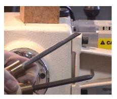
The next step was turning a cap from a cocobolo block to fit into the hole on the base of the ornament. He cut a 3/8th circular hole in the tip of this cap to receive the tenon of a icicle finial which he would turn later. A key step in turning the cap was to cut the face concave inward that would abut against the base of ornament. This was to insure a tight fit against the surface of the ellipsoidal body of the ornament. He also scored two grooves on this same surface to trap any excess glue.
