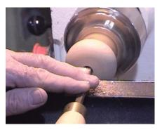
With the base cap completed and glued to the body of the ornament, Joe then turned a cap for the top from the same block of cocobolo which was still mounted in the chuck jaws. He followed the same techniques as used for the base cap except that he embellished the exposed surfaces of the top with a spiraling tool. These marks he set off using a parting tool. Before cutting this cap off, he drilled a small hole in its tip to receive the ornament eyelet.
