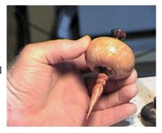
mounted in an Axminster collet chuck. He proceeded to turn the finial using a half inch skew chisel. When sanding the finished finial, he recommended sanding with the grain to prevent sanding marks and then burnishing it with steel wool. Before parting it off, he finished the finial with friction polish. The final ornament was completed by gluing the finial into the hole which had been turned earlier in the base cap.
