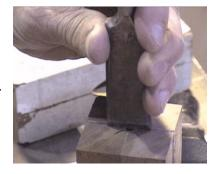
uses the roughing gouge to knock off the edges. He uses a parting tool to make a tenon so he can attach it to his chuck. He uses a cup center on the footstock so it doesn't split the block at the center.
