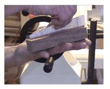
John sketches out the design on a piece of paper, folds the paper in half lengthwise and then cuts ½ of the pattern with an Exacto knife. The pattern is then placed on the flat side of the block and lines drawn across the block.
