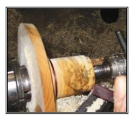
Once the main body of the hat is cleaned up and a rim for the "hatband" is left on, then a piece of Rosewood is held and burnished onto the band for a contrasting color. As the Rosewood heats up it transfers the oils and color to the "band". You can just see the Rosewood stick in the lower right hand corner.
