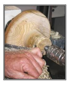
A Tenon is also turned on the small end to enable chucking in a jaw chuck later on.
