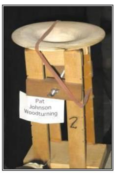
Once the hat was finished turning then it came time to clamp it up for final shaping. As the wood dries this jig compresses the crown and body to give it an oval shape. The threaded rod and wing nut supply the pressure for this. The rubber bands also curl the brim to give it that cowboy hat shape. Only one rubber band is shown in this picture, and normally you would have at least two looped around the brim of the hat and down to the notches in the jig.
