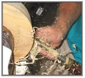
Pat places the truncated conical blank on a screw chuck with the big end toward the chuck. This enables him to turn the brim and crown to rough dimensions and leave no trace of the mounting as the screw enters the waste wood inside the hat.
