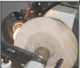
When the blank is turned around and placed in the jaw chuck, the tailstock is brought up and placed in the hole left from the screw chuck. Then a light is strategically placed so as to shine through the brim. As the brim is brought down to a thickness of 3/32nds you
