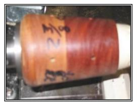
Here is a picture of the jamb chuck that Pat uses for these mini-hats. It is hollow and seems to be mounted on a hollow face plate as well. The reason for this is that a light on a hollow rod (for wiring) will fit up through the jamb chuck to light the interior of the hat to enable turning it down to finished size without removing it to measure thickness.
