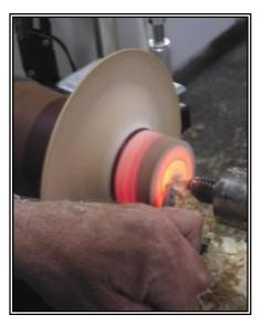
The hat is then reversed once again and placed on the jamb chuck and the light placed inside the hat. The tailstock is once again placed in the center of the Tenon that was left in the first steps.
